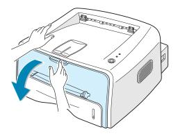
**2** Push the toner cartridge down and remove it from the printer.
